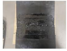
Once the splice is fully sealed, or the fastener is fully covered, leave to cure for the recommended times before restarting belt operation. (see back of brochure)
