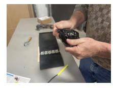
Mix by kneading and squashing the resin pack together until it starst to warm up (2-3 min).
