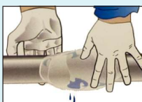
Smooth the Eli-Wrap with wet gloves
